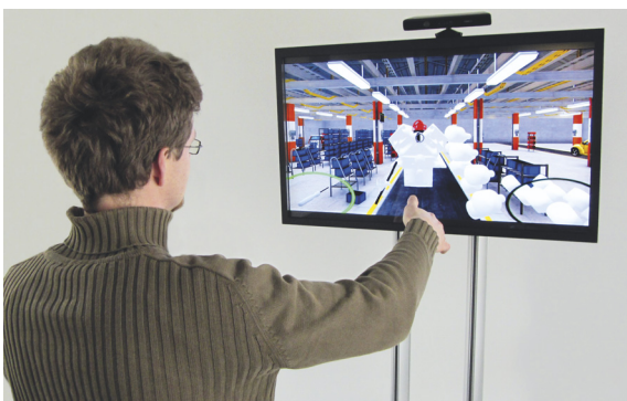
VISTRA training simulator user during assembly of a motorblock
