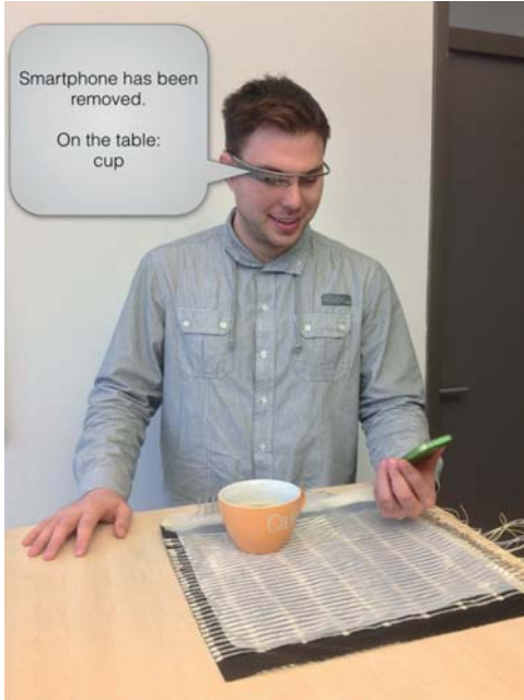
Fabrics with integrated sensors can identify objects based on form and weight.
