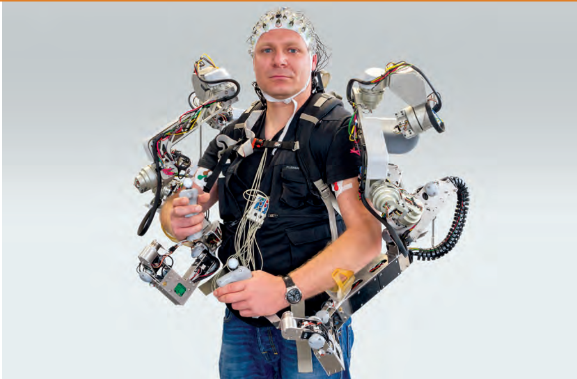
The upper body exoskeleton developed in the previous project Capio for remote control of robotic systems was further developed in RECUPERA-Reha for use in rehabilitation.
