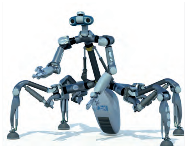
The D-Rock approach demonstrates the effectiveness of using the 6-legged Mantis walking robot developed in project LIMES.
