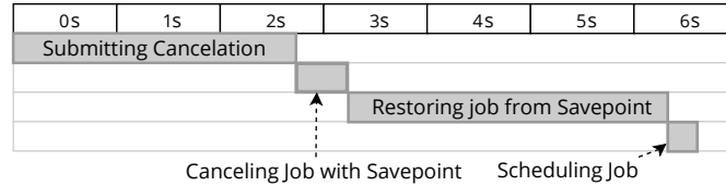
(a) Event timeline for canceling and restoring the stateful map job via a savepoint
