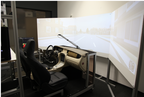
Figure 4: Data capture setup with a Kinect AZURE fixed at the front of a driving simulator.
