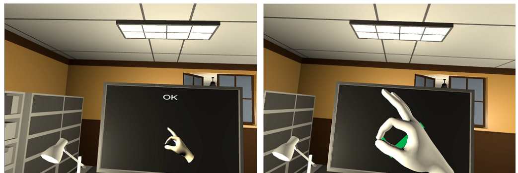
Figure 7. Experiment part one. A gesture is displayed to the participant (left) that should then be imitated (right). This test is to ensure that gestures can be recognized correctly.
