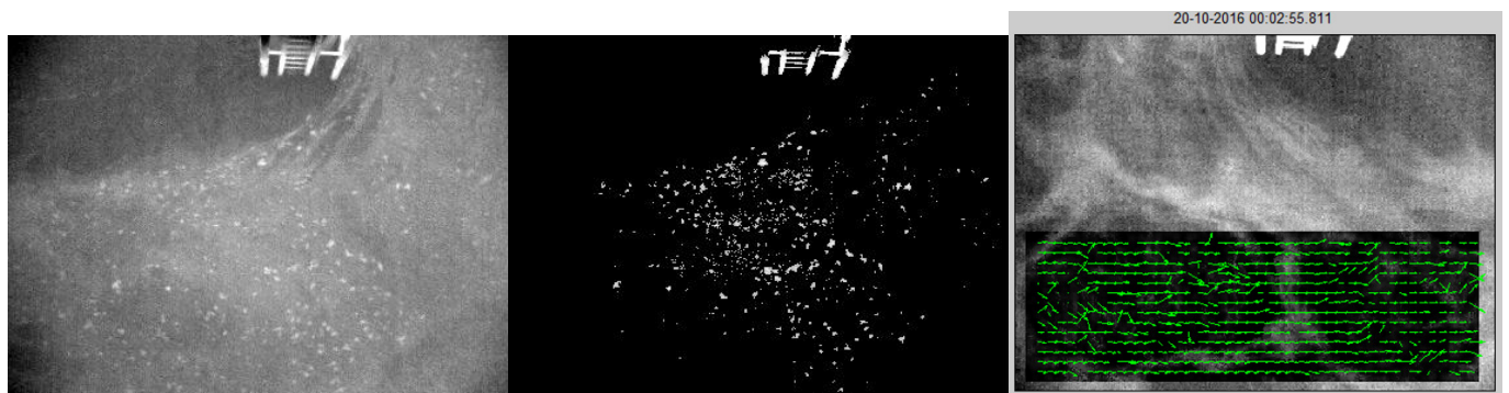
Fig. 4. Left and Center: Shows the comparison between a temperature matrix as a grayscale image from the infrared camera (unprocessed) and the result after image pre-processing with perfect quality. It can be seen that the tracer points become highlighted and segmented, but minimal noise remains in the background, which can lead to higher standard deviations in the LSPIV analysis. Right: Another IR scene during darkness around midnight with region of interest in front of the observation platform, for a long-term observation of undisturbed sea surface current conditions, with superimposed LSPIV vector field
