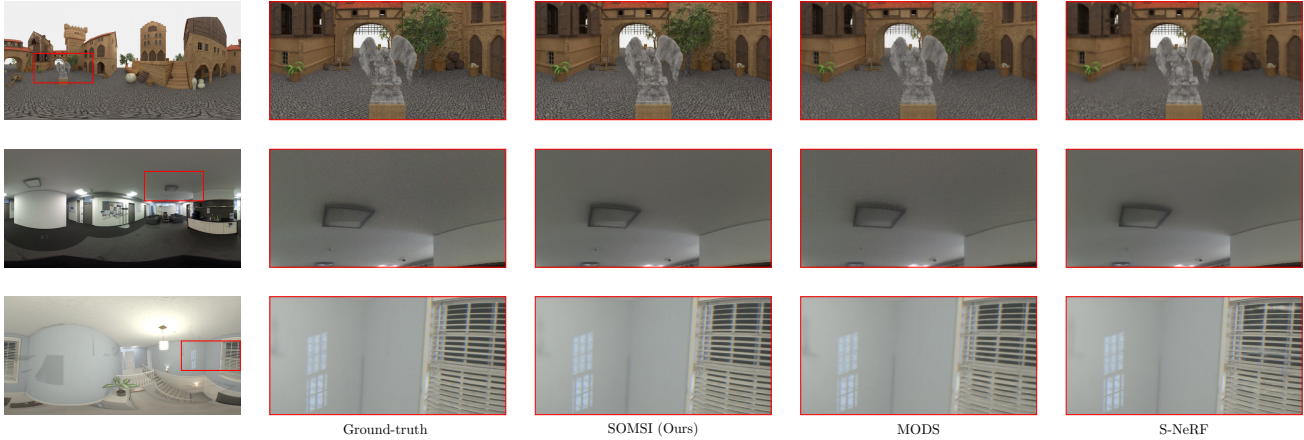
Figure 4. Sample visual results. Novel views on the Sea Port (row-1), Coffee Area (row-2) and Residential (row-3) datasets. Coffee Area is a real dataset captured with Ricoh-Theta-S camera, while the rest are synthetic. In the first row, MODS produces blurred images and struggles with thin structures. S-NeRF creates images with even less details than MODS (see the cobblestones) and far away objects (eg. the tree beyond the gate) are not well reconstructed. Specular reflections (2nd row) and thin structures (3rd row) are better captured with our method. For a better visualization, we encourage the reader to zoom-in on the insets.
