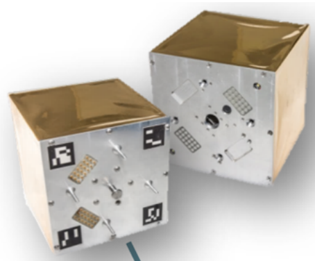
Fig. 7. The Electro Mechanical Interface (EMI) attached to standardized 1U payload item container
