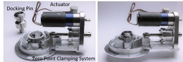
Fig. 4. Locking mechanism of EMI-MOD, opened (left) and closed (right)
