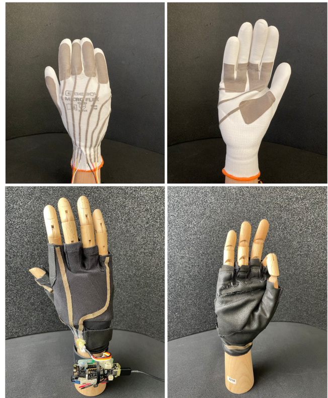
Figure 3: Downstream application for tracking hand and finger movement using smart capacitive sensing gloves
