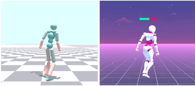
Figure 19: Left : Ragdoll simulation model. Right : Re-targeted visualization model. Our framework is used to learn fatigued movements for a 28 degrees-of-freedom humanoid character. Pink tints indicates fatigued areas ( left ). The color of the rigid body corresponds to the fatigue of its parent joint (e.g. lower leg corresponds to the knee). The health bar indicates the current average residual capacity ( right ).
